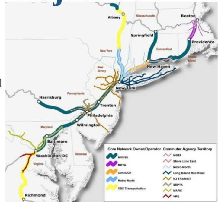
Figure 1: Map of Northeast Corridor rail infrastructure owners and passenger rail operators (Source: NEC Infrastructure Master Plan Working Group 2010)
